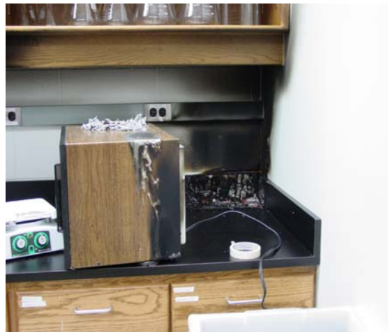
Fire in HSC lab affecting a microwave and an unattended hotplate
