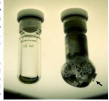
°C, softening the thick glass wall. Fortunately there was no explosion, because the O-ring had cracked open enabling the pressurized contents to be vented.
